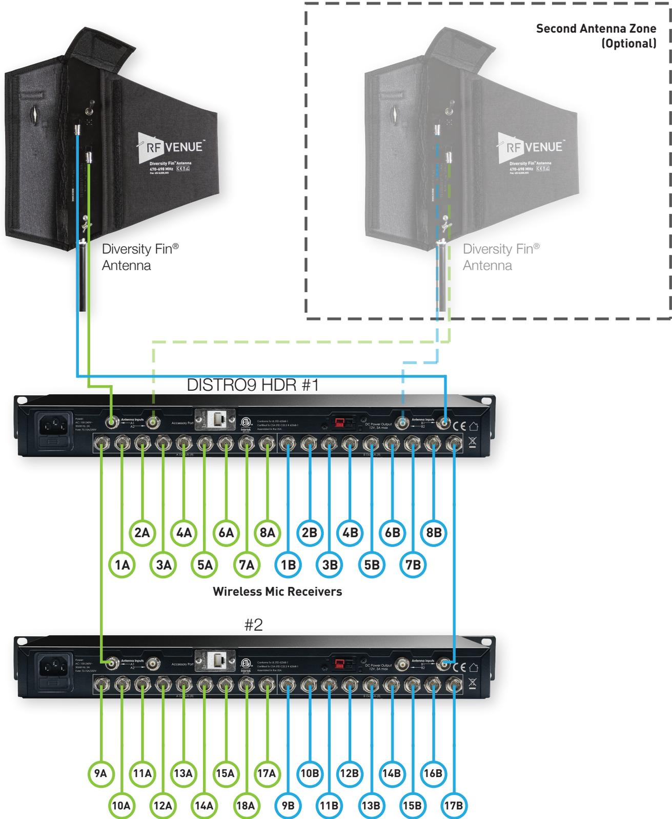
\*DISTRO9HDR #1 (Master) can feed signals to up to 9 additional DISTRO9HDRs. Each connected DISTRO9HDR can feed up to 9 receivers.
